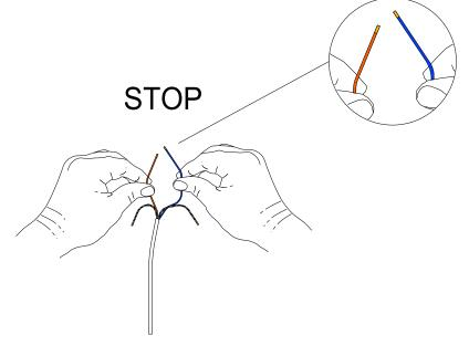
If the Art goes Down, connect and hold the Orange and Blue wires together until the Art jogs up and down. The direction is now reversed.
