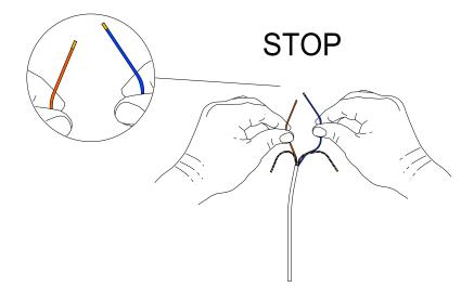
To comfirm the end limits, hold the orange and blue wires until the art jogs, now the end limits are set.
