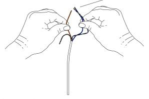
Connect the Orange, Blue/white and blue wires then release once the art will start to move up. the art will stop at its upper limit.
