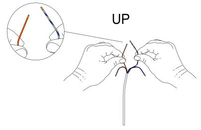
Connect the Orange and the Blue/White wires together, if the Art rises, go to "Adjusting end Limits",
