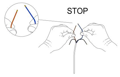
Connect the Orange and the Blue wires to stop the art at the bottom position, you can adjust by going up or down using the right combination
