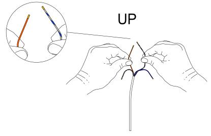
Connect the Orange and the Blue/White wires together until you reach the desired position.
